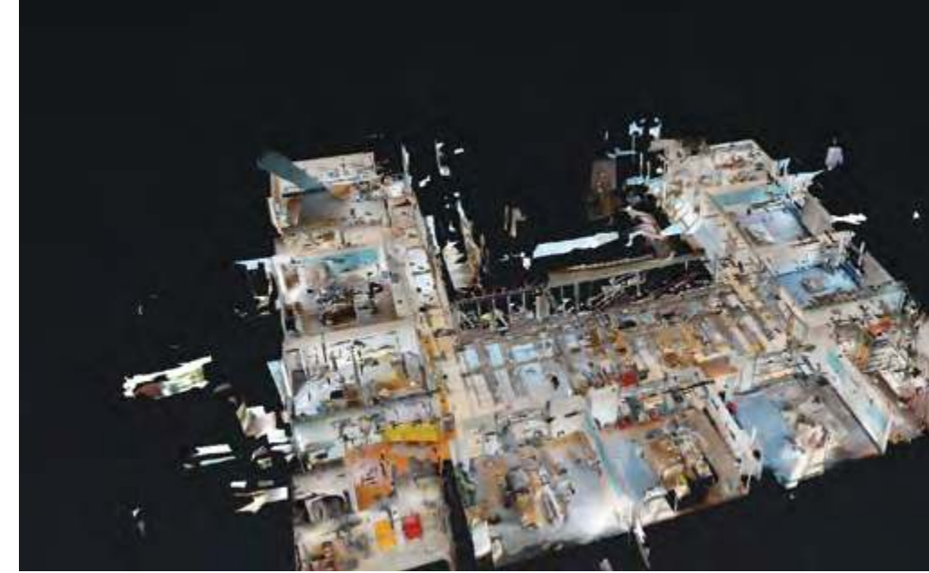
△ Matterport scans create a 3D overview users can navigate through
