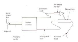
Ground lead can be to the building steel or cable connecting work piece to building steel.
