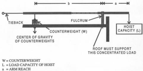
b = BACKSPAN DISTANCE (Distance between the fulcrum point and the center of the counterweights)
