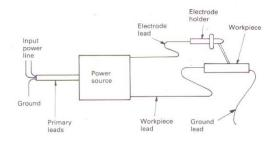
Ground lead can be to the building steel or cable connecting work piece to building steel.
